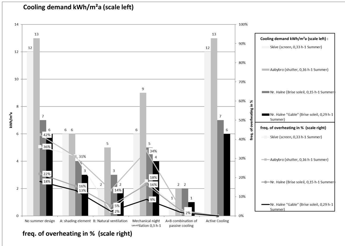
Figure 3: A brise soleil is designed to shade the solar angles, which cause most overheating. It provides a fixed cooling effect of approx. 3 kWh/m<sup>2</sup>, which reduces the cooling demand by natural ventilation by approx. 50 %.
